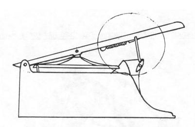
PERIODICALLY, IT MAY BE NECESSARY TO ADJUST THE BAR ATTACHED TO THE HAND LEVER
