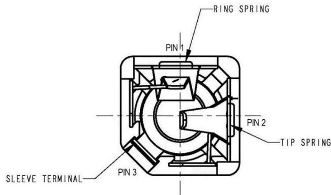
Old wiring assignment: PIN 3 to Terminal 11, PIN 2 to Terminal 10 or 12, PIN 1 is for ground (enclosure). This wiring assignment can only be used with our old style PT1000 sensor.
