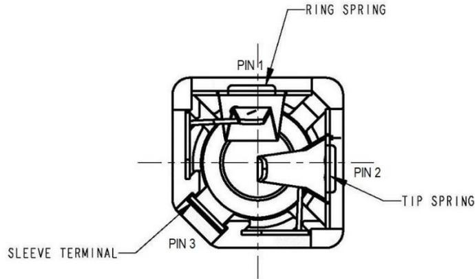
New wiring assignment: PIN 1 to Terminal 11, PIN 2 to Terminal 10 or 12. This new wiring assignment can be used for both old style and new style sensors.
